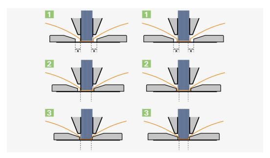
In contrast to conventional perfect binders (left 1-3), the pressing on Muller Martini perfect binders is carried out symmetrically (right). The front and rear pressing plates reach the book block synchronously (2) and press simultaneously (3), resulting in angular and stable book spines. The symmetrical pressing motion is designed to produce beautiful book spines with a wide variety of papers and covers in just one pressing operation.
